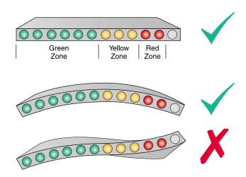
Also included is a rigid plastic housing for use on flat surfaces. Choose your mounting location, making sure that it is clearly visible and doesn't interfere with the function of the motorcycle. The mounting surface must be clean and free from grease. Locate your RevLight with the contact pad supplied. Gently heat the adhesion area to make a stronger bond. Allow 24 hrs for the adhesive to mature fully.
